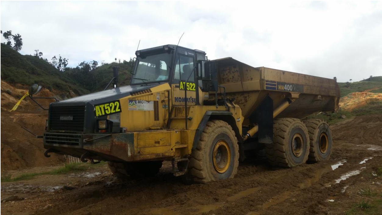
Komatsu HM400 40t articulated tip truck upon arrival at Edie Creek Mine
